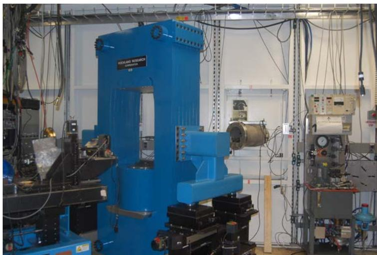
*Figure 1: The 1000 ton press at beamline X17B2 of the National Synchrotron Light Source. This apparatus is used for high-pressure studies of rheology, elasticity, and equations of state of mineral and rock samples at high P&T.*
