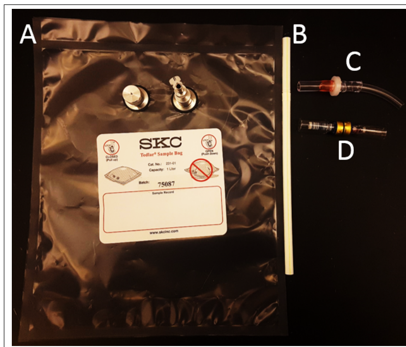
Figure 2.1: Components used in every breath kit. A) 1.5L Tedlar breath collection bag, B) Mouth piece, C) 0.22 \mu\text{m} filter, D) Thermal desorption tube (TDT)
