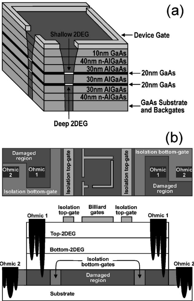
FIG. 1. (a) Schematic representation of the double-layer billiard. The gate widths are 100 nm. (b) Schematic representation of the technique used to achieve independent electrical contact to the two billiards (after Ref. 13).
