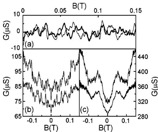
FIG. 2. (a) An overlay of FCF traces (with classical backgrounds removed and for  $B > 0$  only) from the deep (thin line) and shallow (thick line) billiards for  $n=2$ .  $G(B)$  traces for the shallow (upper traces) and deep (lower traces) billiards at (b)  $n=2$  and (c)  $n=8$ . Shallow billiard traces in (b) and (c) are offset by 20  $\mu S$  and 5  $\mu S$ , respectively, for clarity.
