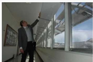
The solar awnings redirect light from the outside using a light bar that reflects sunlight onto the building's ceiling. (Photo courtesy of Oregon BEST)
