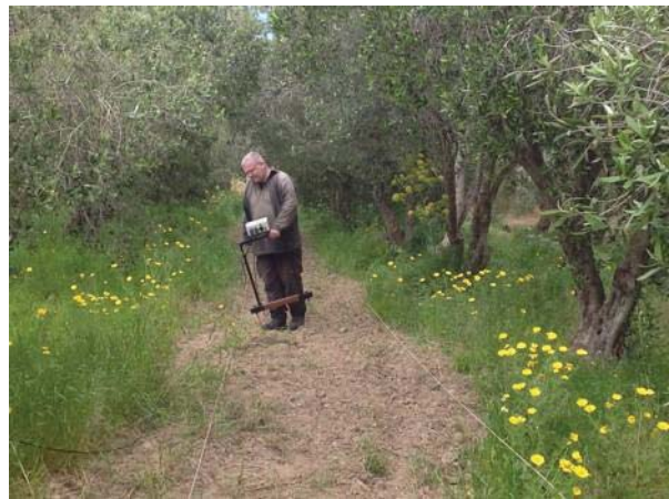
Figure 2: Resistivity survey at Ggantija monument.
