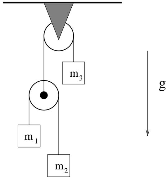
Consider a pulley set-up with three masses as shown. The axle of the upper wheel is fixed, while the lower wheel is suspended from the upper string. Assume that there is no slack in the strings at any time.
