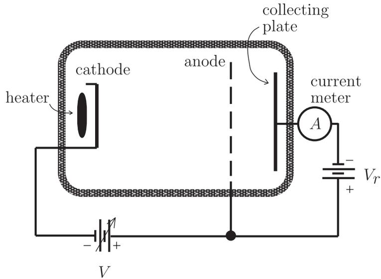
The apparatus depicted above was used in 1914 to study the collisions of electrons with atoms. The chamber is filled with mercury vapor at low pressure. Electrons are emitted thermally at the heated cathode on the left. A variable voltage,  $V$ , is applied between the cathode and a slotted anode. Another voltage of opposite polarity,  $V_r$ , is applied between the anode and an electron collecting plate. The current,  $I$ , between the cathode and the collecting plate is measured by a meter.
