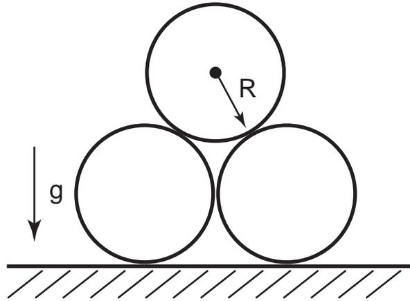
Three identical wooden cylinders of mass  $m$  and radius  $R$  are placed on a horizontal cement floor in a uniform gravitational field of acceleration  $g$  as shown. Find the minimum value of the coefficient of static friction  $\mu$  between the cylinders and the floor such that there is neither translational nor rotational movement.
