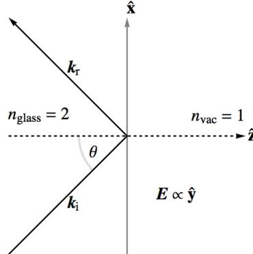
The incident wave: (i) propagates through the glass in the  $xz$  plane; (ii) is linearly polarized in the  $y$  direction; and (iii) travels at angle  $\theta$  with respect to the normal direction  $\hat{\mathbf{z}}$ , to the glass-vacuum interface,
