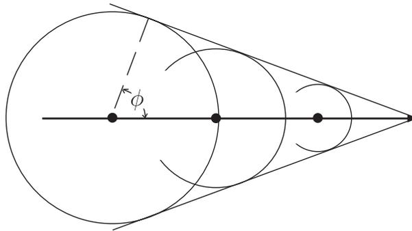
When an electric charge moves through a medium at a speed greater than the wave velocity of light in the medium,  $c/n$ , the charge will radiate. This is Cerenkov radiation, illustrated by the application of Huygen's principle in the figure above.
