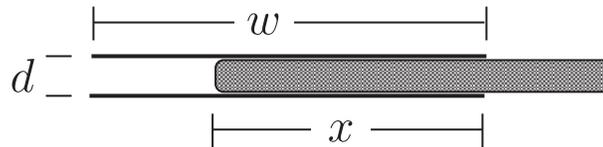
b) A dielectric sheet with dielectric constant  $\epsilon = \epsilon_0\epsilon_t$ , width  $w$  and thickness  $d$  is inserted between the plates to a distance  $x$  (with  $x < w$ ). Calculate the capacitance  $C$  and the energy  $E$  of the system.
