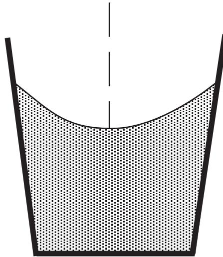
A bucket of water spins about the vertical axis with angular velocity  $\omega$ . When the water has reached a steady state, what shape does the surface of the water take? That is, find the height  $z$  of the water as a function of  $r$ , the distance from the axis.
