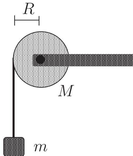
A cord is wrapped around a uniform disk of radius  $R$  and mass  $M$ , which is mounted on an axle supported in fixed, frictionless bearings. A mass,  $m$ , is suspended from the cord.
