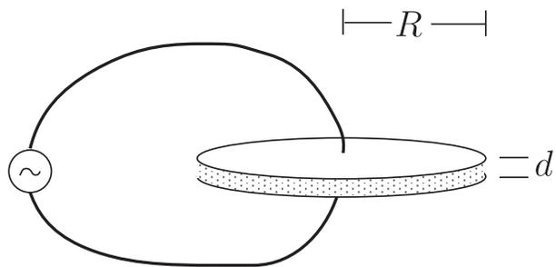
A parallel plate capacitor consists of metal disks of radius  $R$  separated by a gap  $d$ . The material between the plates has conductivity  $\sigma$  and dielectric constant  $\epsilon$ . Assume that  $R \gg d$  so that fringing fields can be neglected. The plates are connected to a generator which provides an oscillating emf given by  $V(t) = V_0 \sin(\omega t)$ .
