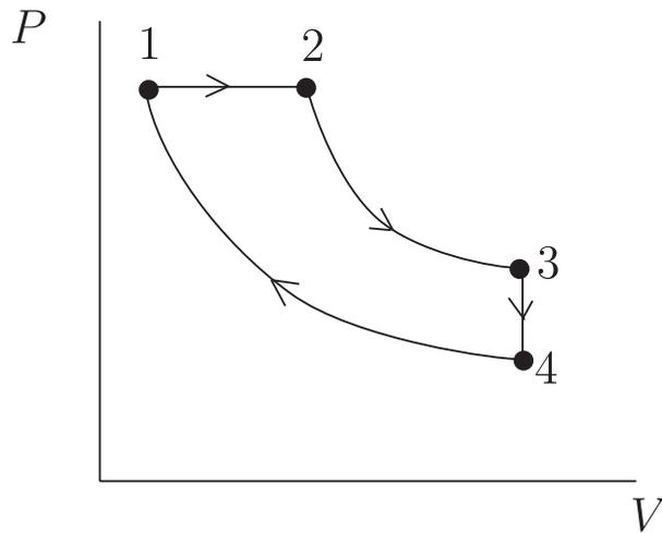
Consider a heat engine running on the cycle shown above. One mole of ideal gas with specific heats  $C_V = 2R$  and  $C_P = 3R$  starts at point 1 with initial temperature, volume, and pressure  $T_1$ ,  $V_1$ , and  $P_1$  respectively. The four steps in the cycle are all reversible. This problem concerns only the first step, which consists of an isobaric (constant pressure) expansion to  $V = 4V_1$ .
