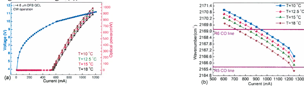
Figure 2: 2(a) LIV curve of a 4.61 \mu\text{m} RT, CW, DFB-QCL from Center for Quantum Devices, Northwestern University; (b) DFB-QCL current tuning at different operating temperatures.
