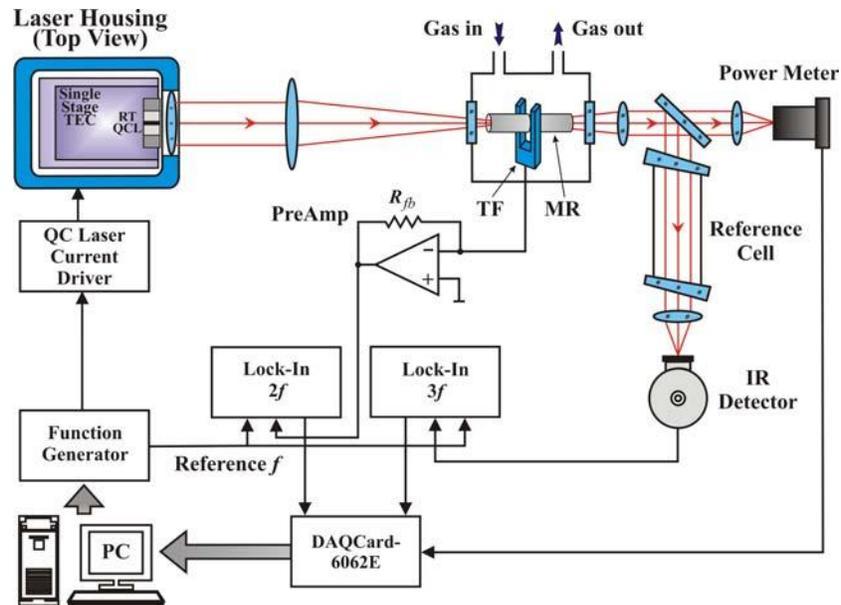
Fig. 3. QEPAS-based ammonia sensor architecture.
