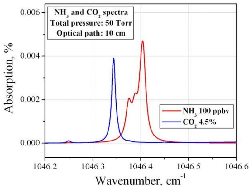
Fig. 2. HITRAN-based simulation of absorption spectra for  $\text{NH}_3$  (100 ppbv) and  $\text{CO}_2$  (4.5%) within the QCL tuning range.  $\text{N}_2$  is used as the diluting gas.
