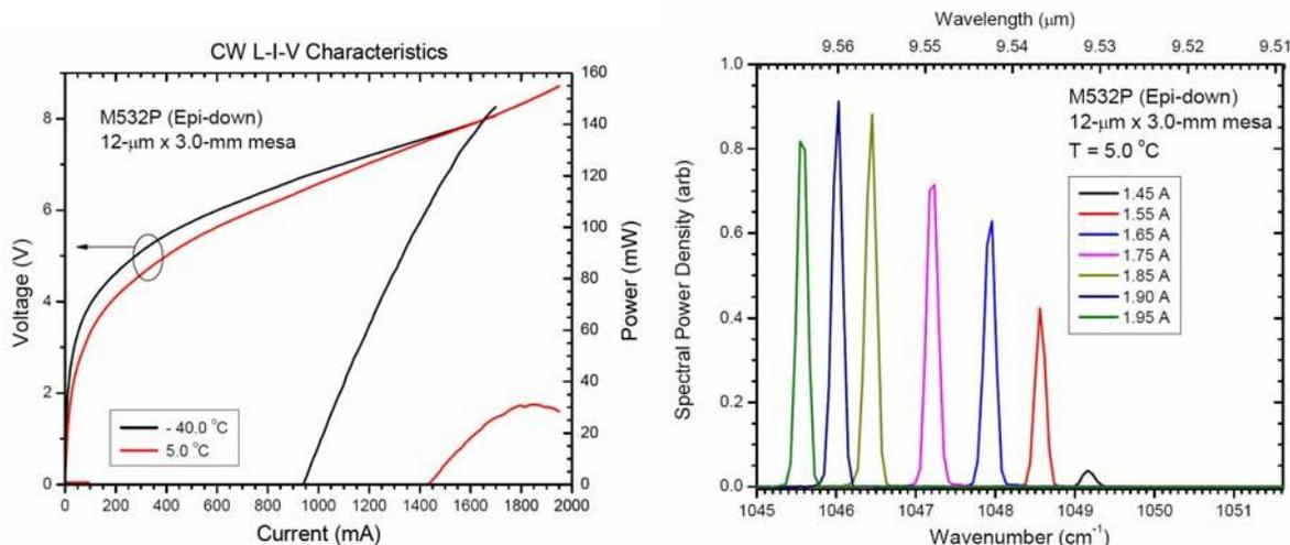
Fig. 1. Power, V-I and spectral characteristics of the CW DFB QCL (Maxion Technologies, Inc., Model # DQ9-M532P)
