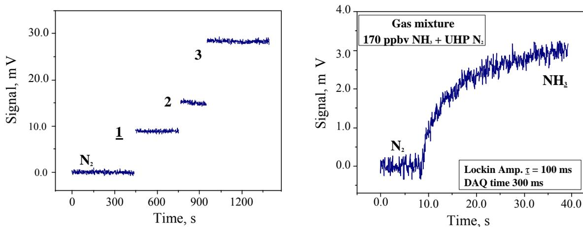
Fig. 4. Sensor performance. Left plot: step concentration measurements were made using a gas standard generator (1 – 300 ppbv, 2 – 500 ppbv, 3 – 1000 ppbv). Right plot: temporal sensor response to the concentration change.
