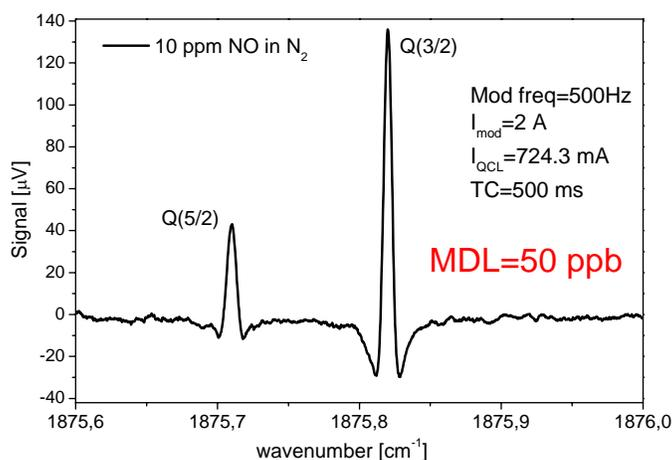
Fig. 3. Faraday rotation spectrum of NO Q(3/2) transition at  $1873.8\text{ cm}^{-1}$ . Minimum detection limit for this measurement was 50 ppb in time constant of 500ms.
