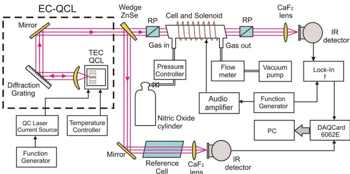
Fig. 1. Schematic configuration of the setup used for Laser Faraday Rotation Spectroscopy of NO.
