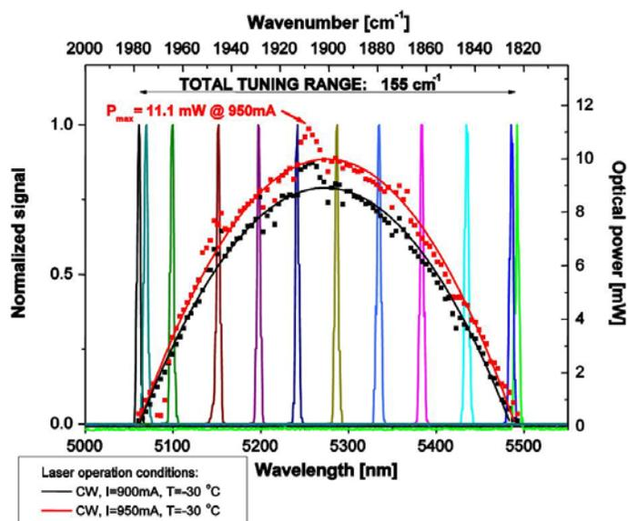
Fig. 2. Wavelength tuning range and corresponding laser power for a 5.2  $\mu\text{m}$  EC-QCL.
