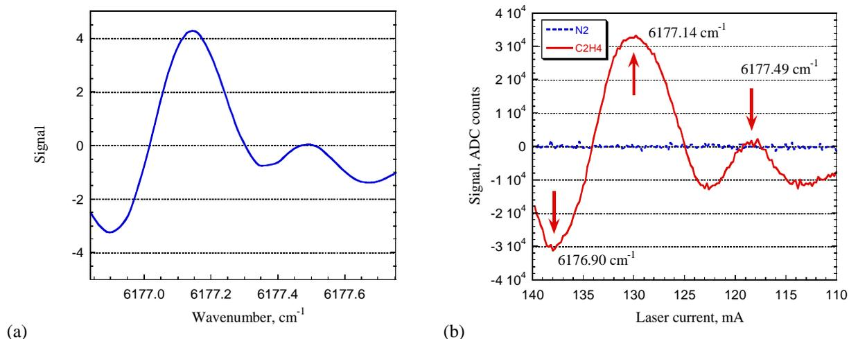
Fig. 2. (a) Simulated  $2f$  signal covering the spectral range utilized for the QEPAS based  $\text{C}_2\text{H}_4$  sensing; (b) Actually recorded QEPAS signal for the same spectral region: solid line – 101 ppmv  $\text{C}_2\text{H}_4$ , dotted line – pure nitrogen. Data acquisition time per point is 5.6 s.
