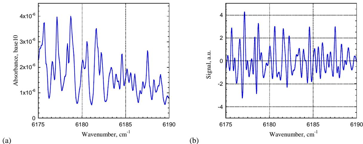
Fig. 1. (a) A fraction of FTIR spectrum from the PNNL database covered by the tuning range of the available DFB diode laser; (b) simulated  $2f$  wavelength modulation spectrum assuming a  $0.20\text{ cm}^{-1}$  WM amplitude and neglecting residual amplitude modulation (RAM).
