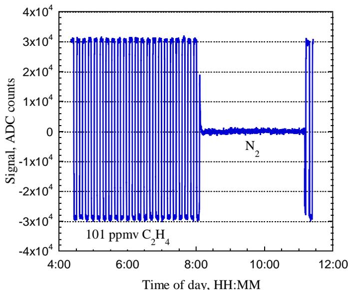
Fig. 3. Continuous monitoring of QEPAS signal (101 ppmv  $C_2H_2:N_2$ ) with the laser wavelength alternately tuned to the  $6177.14\text{ cm}^{-1}$  positive or  $6176.90\text{ cm}^{-1}$  negative peaks in the  $C_2H_2$  2f absorption spectrum. From ~8:10 to 11:10 the sensor was flushed with pure  $N_2$ , while switching of the laser wavelength continued at the same rate. Data acquisition time is ~11.2 s per point.
