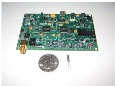
Figure 1: Photograph of sensor board, US Quarter, and quartz tuning fork. This platform was used to measure CO 2 at 2 \mu m using both TDLAS and QEPAS
