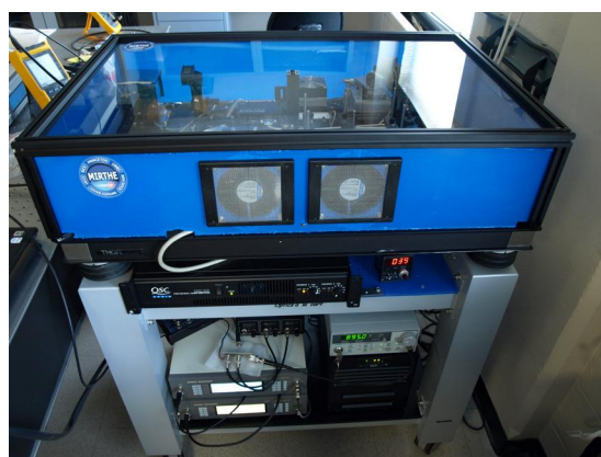
Fig. 5 A transportable prototype FRS NO sensor system
