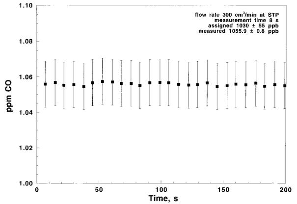
Fig. 7. Measurement of air sample with factory-assigned CO content of  $1030 \pm 55 \text{ ppb}$ . The value measured in the experiment is  $1055.9 \pm 0.8 \text{ ppb}$ , based on the calibration data from Figure 6. Error bars represent the root-mean-squared fit residuals, equivalent to 13 ppb CO.
