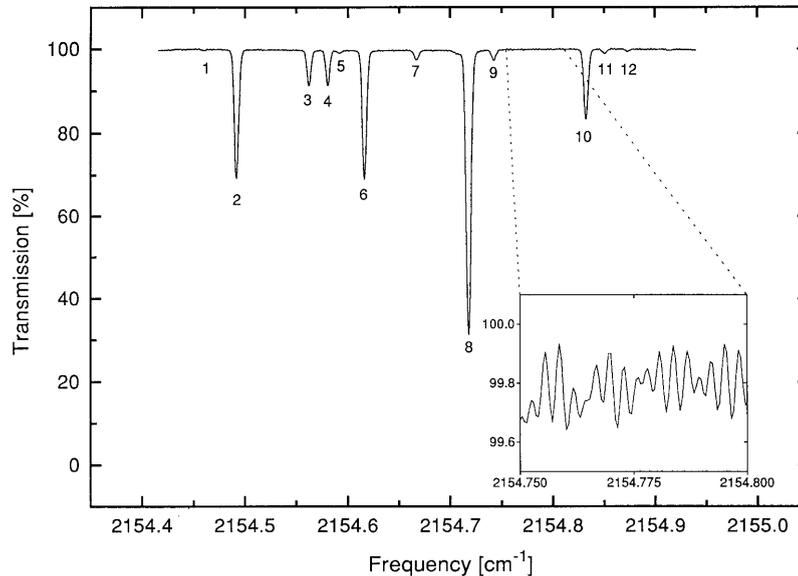
Fig. 4. Infrared spectrum of  $N_2O$  in the multipass cell at a pressure of 2.5 Pa. Table 1 lists the corresponding transition frequencies. The trace is a 512 sweep average, corrected for the amplitude modulation associated with frequency tuning. The inset shows magnified interference fringes due to scattering in the multipass cell, limiting the signal-to-noise ratio to 300.
