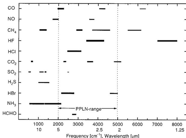
Fig. 9. The range of mid-infrared transitions for various atmospheric pollutants is shown. Data were taken from the HITRAN database.<sup>21</sup>
