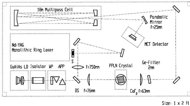
Fig. 1. Diagram of the optical section of a portable sensor for trace gas detection, based on diode-pumped mid-infrared DFG in bulk PPLN. The size of the section is 65 cm × 31 cm × 15 cm. Here WP is a half-wave plate, APP is an anamorphic prism pair, S is a shutter, and BS is a beam splitter.
