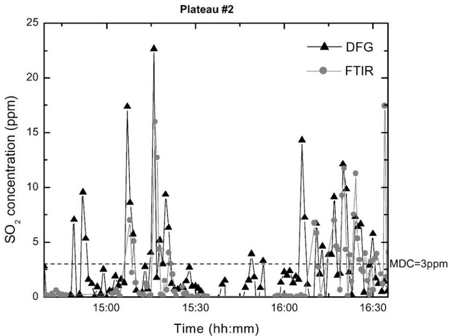
Fig. 7. Measurements of SO<sub>2</sub> emitted by Masaya volcano. Shown are the measured SO<sub>2</sub> concentrations of the extractive DFG-based gas sensor and open-path FTIR gas sensor.
