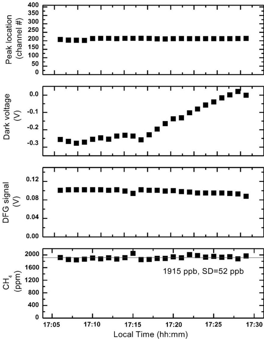
Fig. 4. Measurement of CH<sub>4</sub> at Masaya volcano, Plateau 2, April 14, 2000. Also shown are DFG signal, dark voltage and peak location, indicating a stable, nearly drift free time period. The estimated measurement accuracy is 7%.
