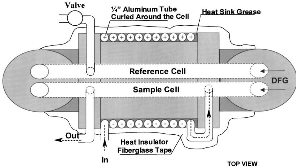
Fig. 8. Dual chamber gas sampling cell for precision isotopic ratio measurements of  $^{13}\text{CO}_2/^{12}\text{CO}_2$ .  $\text{CaF}_2$  windows are at Brewster angle to minimize optical interference.
