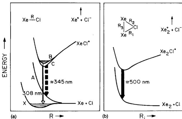
FIG. 2. Simplified potential-energy diagram of the diatomic excimer XeCl and triatomic excimer Xe<sub>2</sub>Cl.
