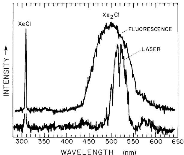
FIG. 3. Fluorescence and laser spectrum of Xe<sub>2</sub>Cl and XeCl ( $B \rightarrow X$ ) of an Ar/Xe/CCl<sub>4</sub> mixture of 6.5 atm, 200 Torr, and 1 Torr, respectively. All intensities are shown in arbitrary units, not corrected for the spectral response of the OMA Model 1205D/01 vidicon detector.
