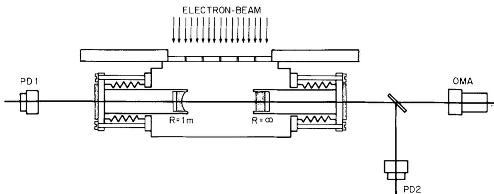
FIG. 1. Schematic of electron-beam-pumped laser cell and associated diagnostic instrumentation.
