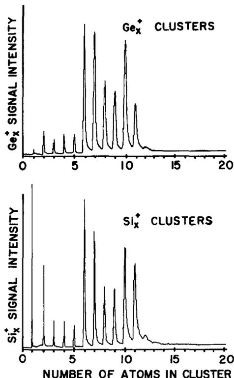
FIG. 2. Time-of-flight mass spectrum of germanium and silicon clusters. The clusters were ionized with a moderate fluence ( $0.5 \text{ mJ/cm}^2$ ) ArF excimer ( $6.4 \text{ eV}$ ). All cluster peaks shown are results of multiphoton ionizations. The right-handed tails on the peaks for clusters containing 6–11 atoms indicate that fragmentation from higher masses contributes to these channels. The instrument is optimized to observe clusters in the size range 6–20.
