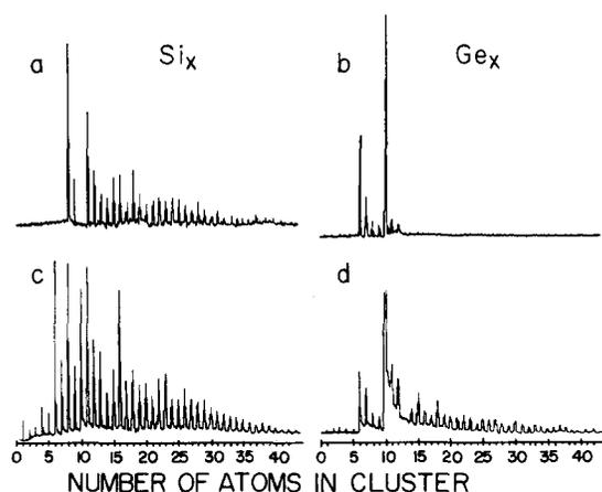
FIG. 5. Time-of-flight mass spectra of clusters ionized by a  $F_2$  excimer laser at  $0.01 \text{ mJ/cm}^2$  (top) and at  $0.2 \text{ mJ/cm}^2$  (bottom) for both silicon and germanium supersonic cluster beams.
