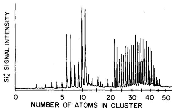
FIG. 3. Mass spectrum of silicon clusters ionized with a low fluence ( $0.05 \text{ mJ/cm}^2$ ) ArF excimer ( $6.4 \text{ eV}$ ). The instrument is optimized to observe clusters in the size range 6–20. Note the onset of one-photon ionization at  $\text{Si}_{12}^+$ .
