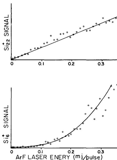
FIG. 4. Dependence of  $\text{Si}_{22}^+$  and  $\text{Si}_6^+$  signals on ArF excimer laser photon fluence. The linear dependence of the  $\text{Si}_{22}^+$  signal indicates a one-photon ionization process, whereas the quadratic dependence of the  $\text{Si}_6^+$  signal indicates a two-photon ionization process.
