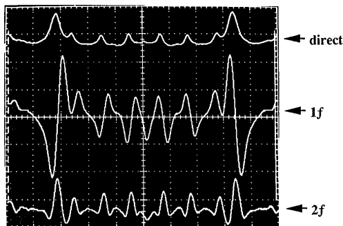
Fig. 3. Direct-absorption (top trace) and wavelength-modulation 1f and 2f (middle and bottom traces, shown on the same vertical scale) spectra of CO 2 in 2.5-m ambient air near 2303 \text{cm}^{-1} recorded with a digital scope. The frequency sweep of 2.5 \text{cm}^{-1} is reversed at the center. The transitions seen here are P(50) (0001–0000), R(26) (0001–0000), P(39) (0111–0110), and R(24) (0001–0000), from left to right in the left half of the figure. 5 Both R transitions belong to 16 O 13 C 16 O.
