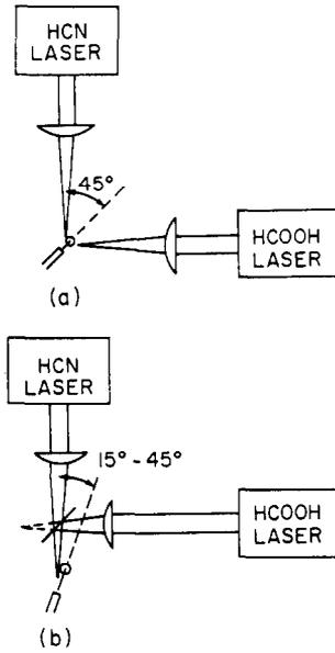
Fig. 3. Duplexing schemes for illuminating the diode with both laser signals. (a) Right-angle coupling resulting from 45° beam direction on a 1-1/4λ antenna. (b) Beam-splitter combiner, using high gain 7-3/4λ long antenna.
