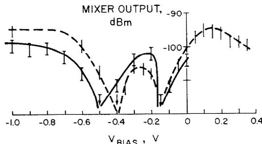
Fig. 5. Rectified signal (video response) and mixer signal output as a function of average d.c. voltage across an  $n$ -InSb diode. The continuous and dashed curves represent two different contacts.
