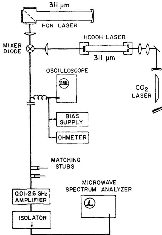
Fig. 1. Diagram of the experimental apparatus, showing the two lasers and the electrical connections to the diode.
