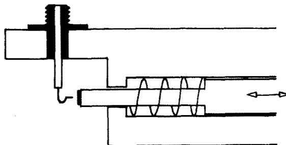
Fig. 2. Detail of the whisker diode, and the diode mount.
