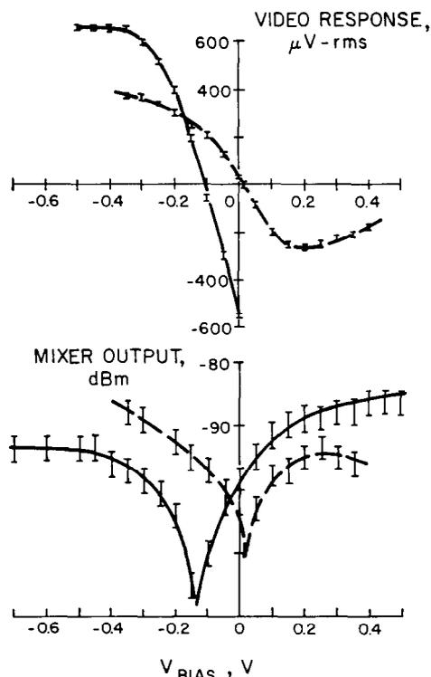
Fig. 6. Mixer output power as a function of bias voltage for a tungsten *p*-Ge diode. Broken and continuous lines represent two different contacts.
