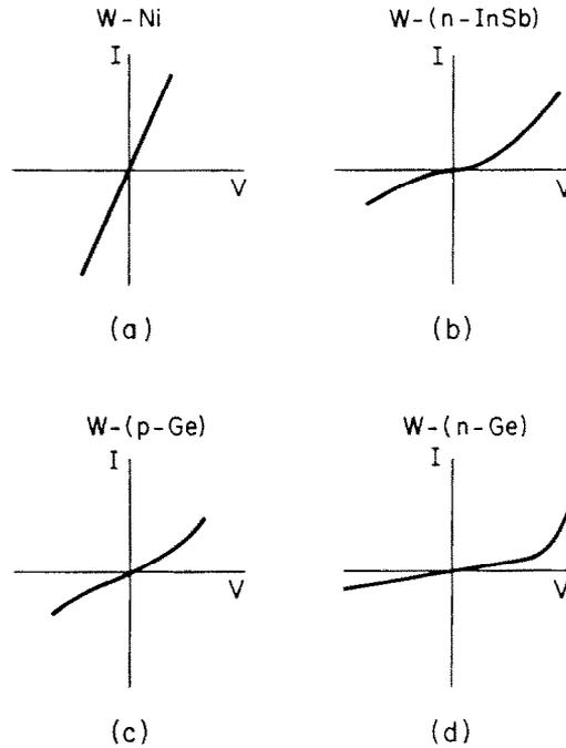
Fig. 4.  $I$ - $V$  characteristics of the 4 diodes studied. All curves are drawn to the same scale.
