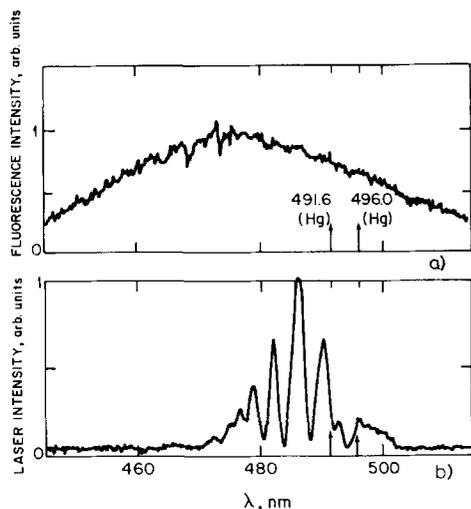
FIG. 2. Time-integrated spectra of (a) fluorescence and (b) laser emission from the  $C_2^3 \rightarrow A_2^3$  transition of XeF (16 Torr Xe, 8 Torr  $NF_3$ , and 600 kPa Ar).
