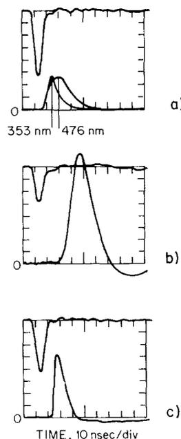
FIG. 1. Time history of e-beam pulse and (a) fluorescence at 353 and 476 nm, (b) lasing at 486 nm, and (c) lasing at 353 nm from a standard mixture of 16 Torr Xe, 8 Torr NF<sub>3</sub>, and 600 kPa Ar; time scale: 10 ns/div.
