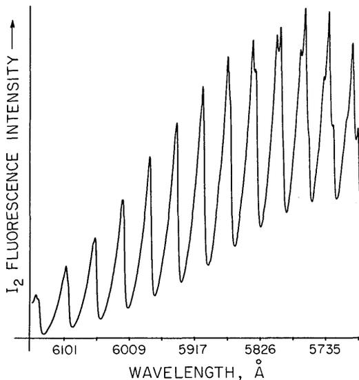
Fig. 5. Low-resolution I<sub>2</sub> fluorescence spectrum from 569 nm to 615 nm; I<sub>2</sub> vapor pressure 0.2 Torr; Rh6G dye laser linewidth = 40 GHz; peak power = 500 mW.
