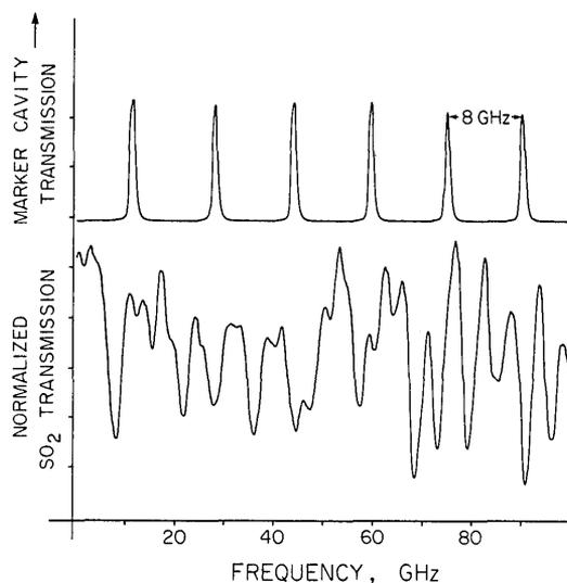
Fig. 8. High-resolution SO<sub>2</sub> absorption spectrum near 305 nm, probe power 0.03 mW, UV scan interval 100 GHz.
