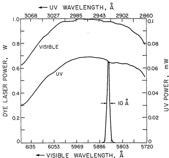
Fig. 4. Typical spectrometer output in visible and UV for a Rh6G dye laser showing effective computer controlled tracking of the dye laser and the orientation of an ADP crystal. Dye laser was operating multimode with 4 W of Ar laser pump power at 5145 Å. Typical scan time of depicted power spectrum is 30 sec.
