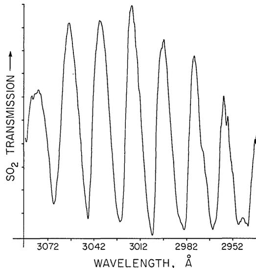
Fig. 7. Low-resolution SO<sub>2</sub> absorption spectrum from 294 nm to 309 nm. SO<sub>2</sub> pressure 2 Torr; cell length 25 cm, peak power 0.05 mW.
