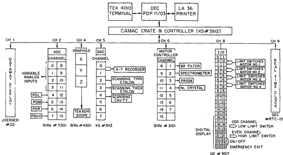
Fig. 3. CAMAC control system for computerized laser spectrometer.
