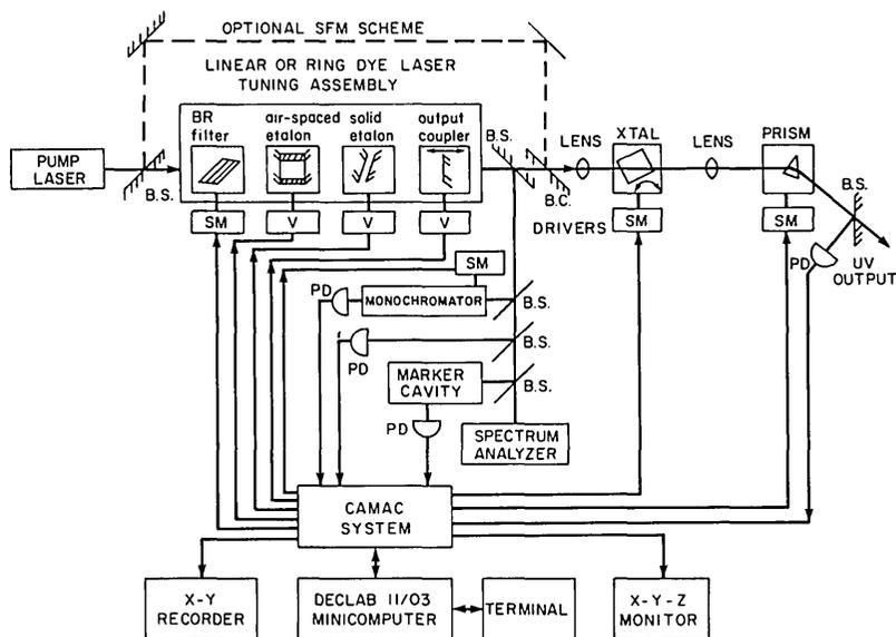
Fig. 1. Schematic of computer controlled visible-UV cw laser spectrometer.
