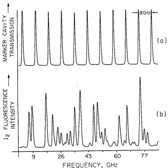
Fig. 6. High-resolution I<sub>2</sub> fluorescence spectrum near 600.2 nm; I<sub>2</sub> vapor pressure 0.2 Torr; Rh6G laser linewidth  $\pm 20$  MHz; probe power 500 mW; scan interval 85 GHz.
