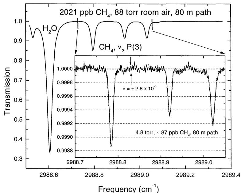
Fig. 4: Room air spectrum of the  $\text{CH}_4$  P(3)  $\nu_3$  ro-vibrational lines at  $P = 88$  torr and 2  $\text{H}_2\text{O}$  lines. The inset is a low pressure  $\text{CH}_4$  spectrum in the same spectral region ( $\sim 87$  ppb of methane in nitrogen)
