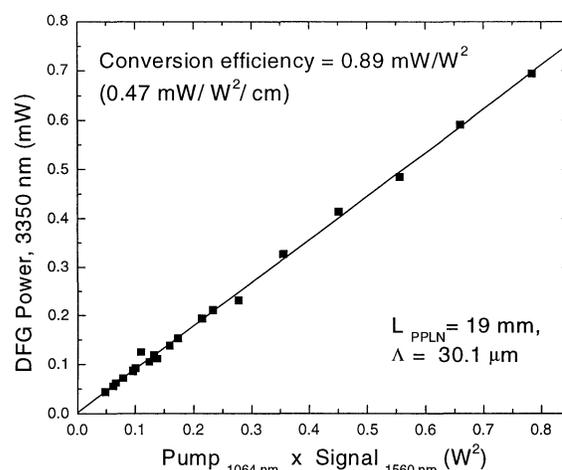
Fig. 3: DFG conversion efficiency
