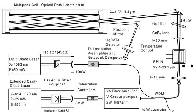
Fig. 1: Optical setup of a fiber coupled widely tunable DFG spectrometer.
