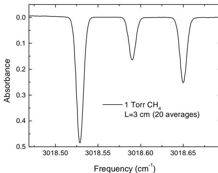
Fig.3: Doppler broadened Q-branch CH<sub>4</sub> spectrum near 3.3  $\mu\text{m}$ .
