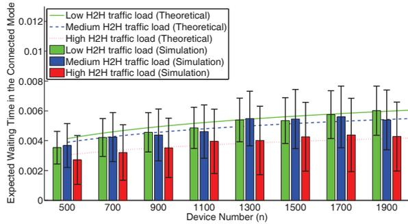
Fig. 5. Expected waiting time (delay) in the connected mode vs. M2M device number under high/medium/low H2H traffic load scenarios with  $\lambda = (30, 35, 40)$  respectively
