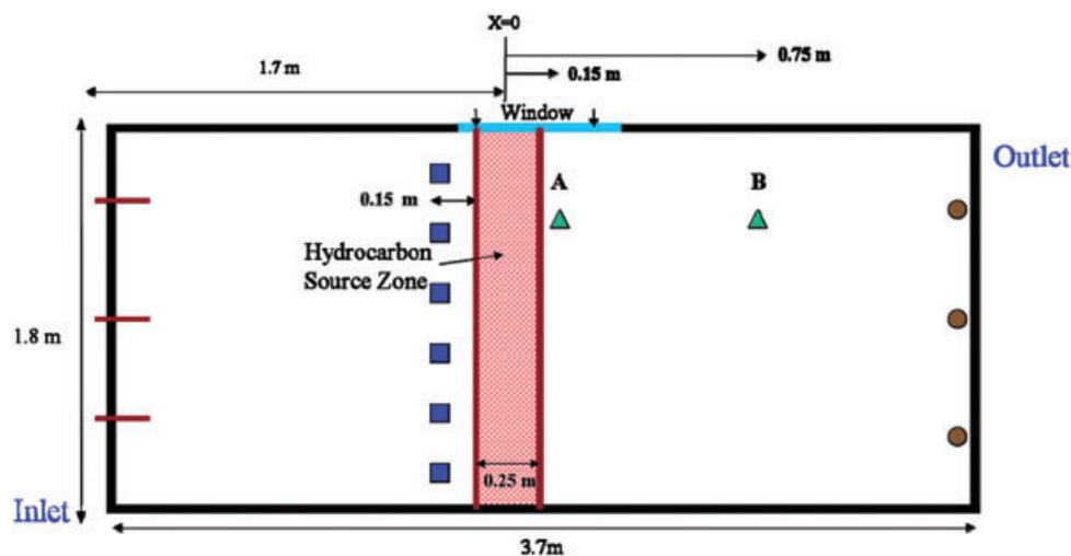
**Fig. 1.** Sampling locations (plan view). Microbial sampling locations are designated by the triangles labelled 'A' and 'B', respectively 0.15 and 0.75 m from the centre of the hydrocarbon source. The six E100 source injection locations 0.3 m up gradient of the mid-point of the emplaced hydrocarbon source zone are represented with squares, and the circles represent outlet well locations.
