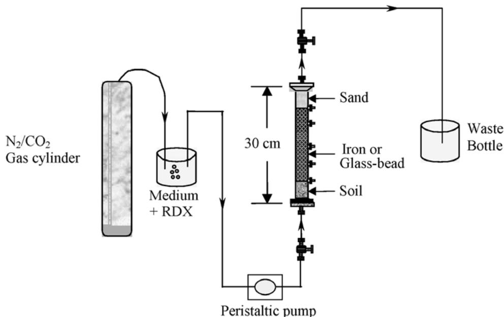
Figure 1. Flow-through columns used to mimic permeable reactive iron barriers.
