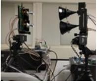
A programmable phased-array antenna in the WiMi testbed at the University of Wisconsin-Madison.
