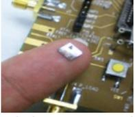
Wireless antenna of the future: 5 mm x 5 mm chip shows the size of antennas in future cell phones.
