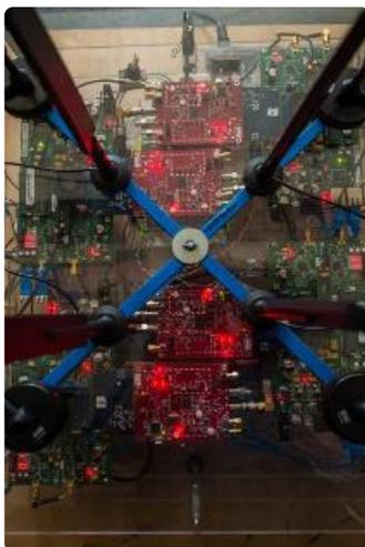
*Rice University's Wireless Network Group has created a multiuser, multiantenna transmission scheme for UHF, a portion of the radio spectrum that could be useful for broadband Internet service in rural areas. Credit: Jeff Fitlow/Rice University*
