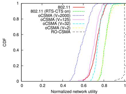
Fig. 9: Cumulative density function of the normalized logarithmic utility attained by different protocols over 100 randomly-generated topologies with 48 flows.
