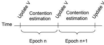
Fig. 3: Alternation of contention estimation and parameter update phases for automatic V adaptation.
