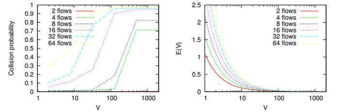
(a) Collision probability as a function of  $V$  and  $F$ . (b) Theoretical bound  $E(V)$  for the optimization error, as a function of  $V$  and  $F$ .
