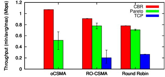
Fig. 5: Results obtained by different protocols in a scenario with competing heterogeneous traffic flows.
