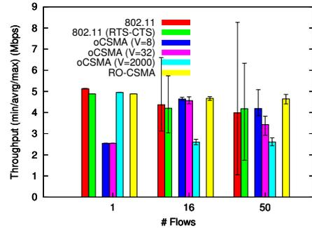
Fig. 6: Per-flow throughput normalized times the number of contending flows in fully connected networks with different sizes.
