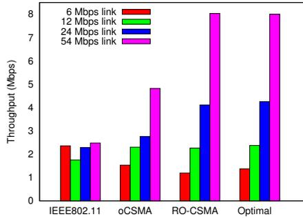
Fig. 4: Throughput distribution attained by different protocols in a scenario with four contending flows and asymmetric link capacities.
