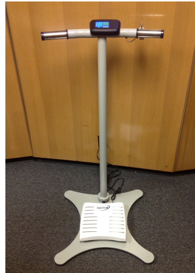
Fig. 1. A full-device view of the Blue Scale, which is used for wireless point-of-care cardiovascular self-monitoring.
