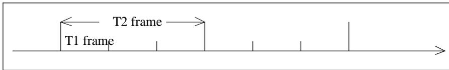
Figure 2: Two levels of framing with  $T_2 = 3T_1$
