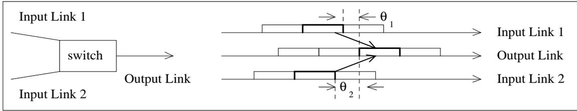
Figure 1: Synchronization between input and output links in Stop-and-Go
