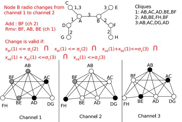
Fig. 3. Example: Derivation of eligibility conditions. There are three channels, each with three cliques. Black/white vertices: Links  $l$  of clique  $j$  with  $F_{l,j} = 1/0$ . Horizontal-striped vertices:  $Rmv$  set. Vertical-striped vertices:  $Add$  set.
