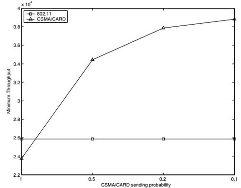
Fig. 12. Minimum throughput vs. RRTS sending probability,  $p_s$ , for CSMA/CARD and 802.11 in topology 2.
