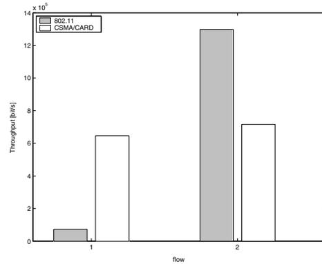
Fig. 6. Throughput of flow  $f_{AB}$  and flow  $f_{CD}$  in the Asymmetric Flows scenario.
