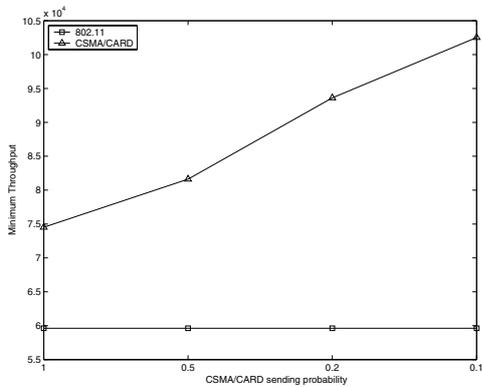
Fig. 9. Minimum throughput vs. RRTS sending probability,  $p_s$ , for CSMA/CARD and 802.11 in topology 1.
