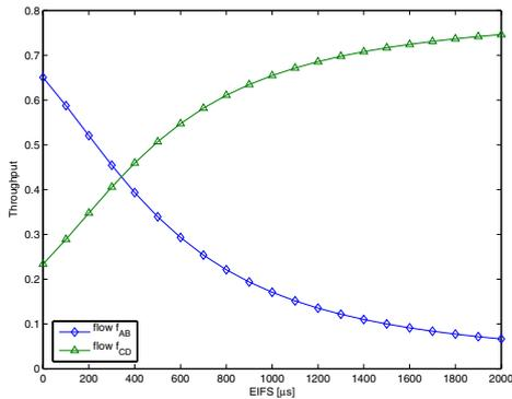
Fig. 5. Throughput of flows  $f_{AB}$  and  $f_{CD}$  vs. length of EIFS.
