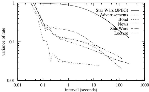
Figure 3: Variance of Rate over Multiple Interval Lengths for Video Traces
