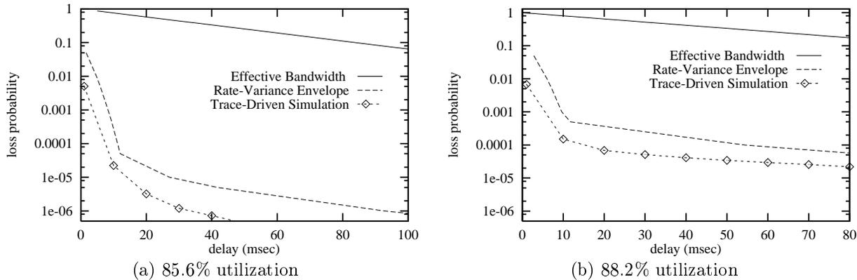
Figure 6: Probability of Loss vs. Buffer Size
