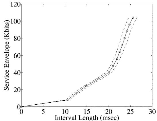
Fig. 4. Service envelope for multiplexed on-off sources.
