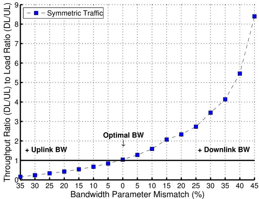
Figure 5.6: Impact of mismatch in optimal bandwidth setting on throughput to load ratio for symmetric traffic.
