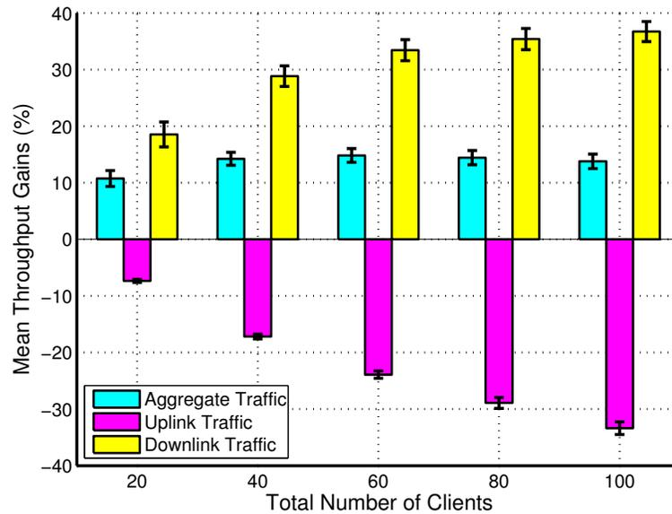
Figure 5.11: Dual Wi-Fi throughput gains over 802.11 with load asymmetry (DL/UL) of 4 for different network densities.
