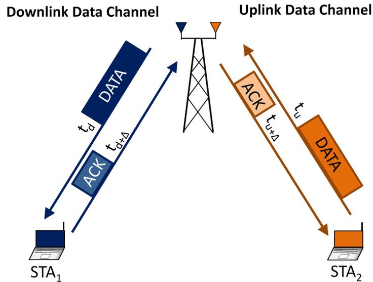
Figure 3.2: Bi-directional Data-ACK communication performed individually and asynchronously in each downlink and uplink data channels. Isolated downlink and uplink data channels, allow simultaneous transmissions even in clique networks.
