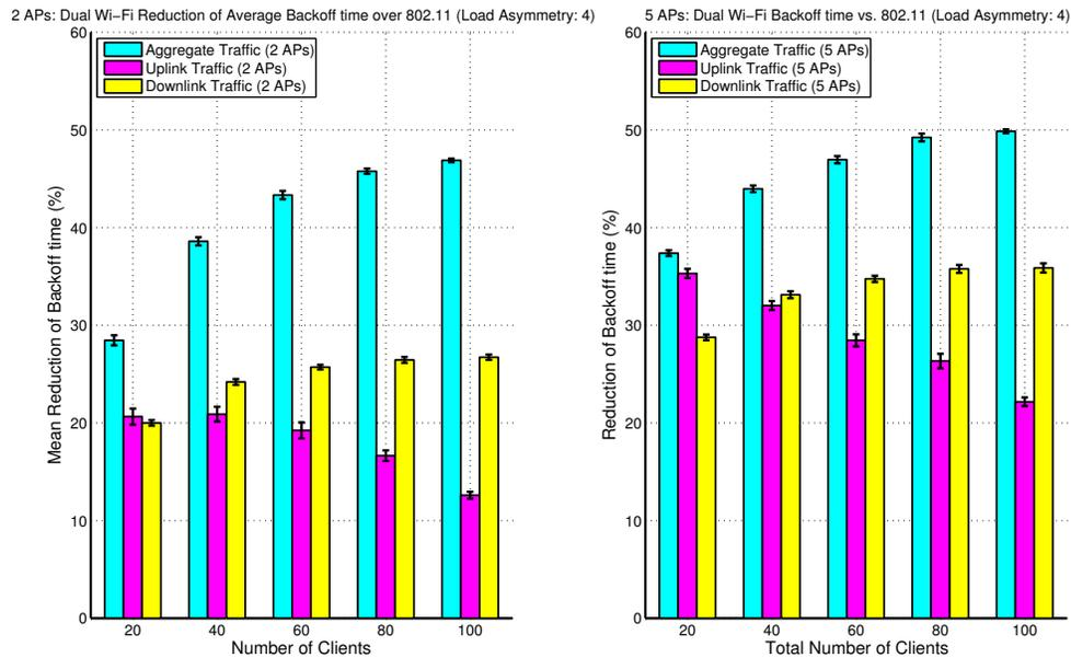
Figure 5.14: Mean reduction of backoff time per successful data transmission over 802.11 with load asymmetry (DL/UL) of 4. Left: 2 in-channel AP topology, right: 5 in-channel AP topology.
