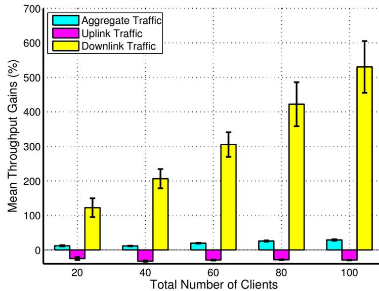
Figure 5.10: Dual Wi-Fi throughput gains over 802.11 with symmetric traffic for topologies with 1-5 in-channel APs.
