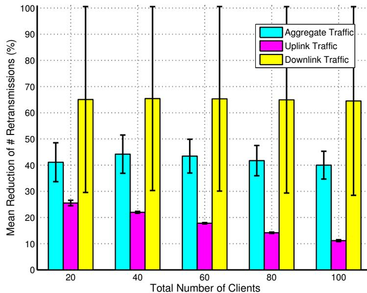
Figure 5.17: Average reduction of number of retransmissions per transmitted packet over 802.11 with load asymmetry (DL/UL) of 4 for topologies with 1-5 in-channel APs.
