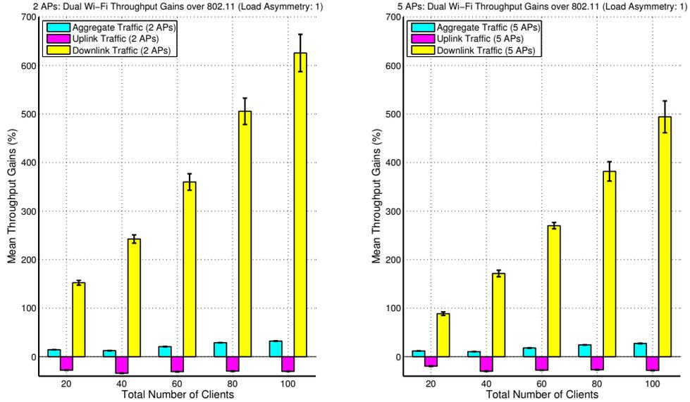
Figure 5.9: Dual Wi-Fi throughput gains over 802.11 with symmetric traffic. Left: 2 in-channel AP topology, right: 5 in-channel AP topology.
