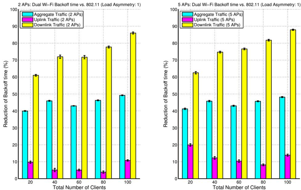
Figure 5.12: Mean reduction of backoff time per successful data transmission over 802.11 with symmetric traffic. Left: 2 in-channel AP topology, right: 5 in-channel AP topology.
