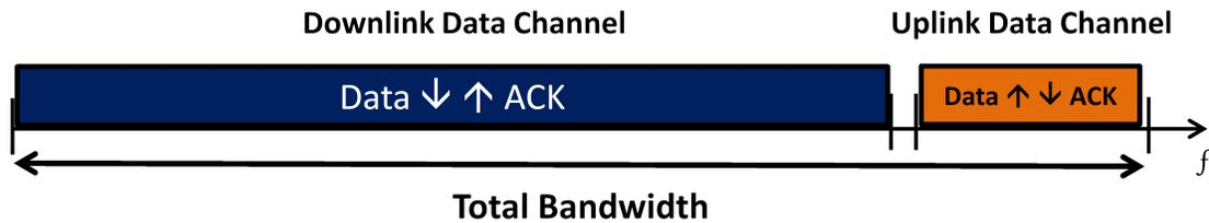
Figure 3.1: Dual Wi-Fi channel architecture: two bi-directional physical channels each carrying a single uni-directional MAC traffic direction, with configurable asymmetric spectrum resource allocation.
