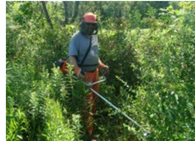
Figure 5. Brush saws are effective tools for vegetation management. The shoulder strap provides a barrier for kickback that would injure the operator. Safety equipment is still necessary.
