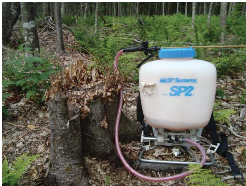
Figure 4. Backpack sprayers are inexpensive and handy tools for applying foliar, basal bark, and cut-stump applications of herbicide. Several brands of sprayers are available. Knowing the correct mixing concentration will reduce waste, minimize unnecessary applications of herbicides, and improve the success of the treatment. The sprayer brand pictured holds approximately 3 gallons, the V_2 used in Formula 2.
