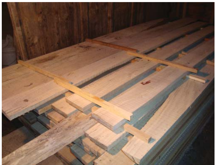
Figure 5. Lumber should be stickered immediately after sawing, ideally as the boards come off the mill. Indoor storage, as illustrated, is ideal if space is available.
