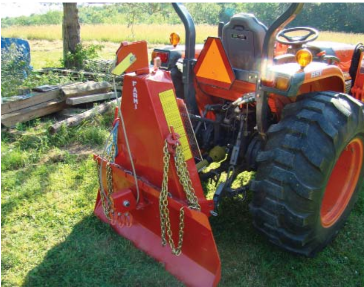
Figure 3. Special attachments for ATV and tractors, shown here with a winch, increase safety and productivity. Care is needed if these types of machines are used for small scale logging.
