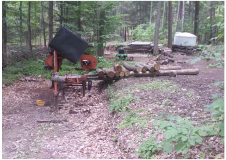
Figure 4. Advance planning will allow arranging logs in a manner to more easily load the sawmill. Creating a cut bank or using a gentle slope makes easy work of loading logs if the sawmill lack hydraulics.
