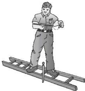
Figure 3. Proper location for inserting temperature probe.
