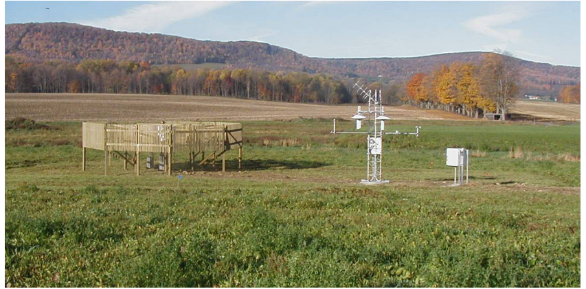
Weather stations around the world have been collecting weather data for more than 100 years. These long-term weather records tell us our climate is changing. US Climate Reference Network stations like this one near Cornell University (Ithaca, NY) provide high quality temperature and rainfall observations.
