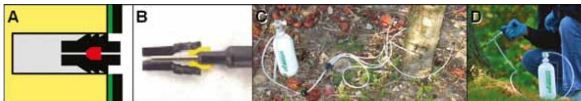
Figure 1. Arborplug ® no. 4 (A) with silicone septum in the injection channel, acting as a one-way valve (red rectangle). Plug cross section showing needle penetrating the white septum during injection (B). Tree I.V. ™ (C) and Quik-jet ® (D) systems used to trunk-inject apple trees (Arborjet Inc., USA).
