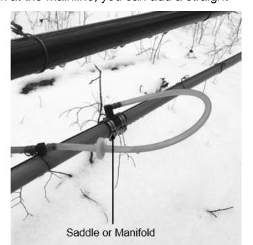
the hole. It is then either and tied or screwed down to create a tight seal. A short loop of tubing is attached to link the end of the lateral line to the fitting on the saddle. Make sure both the free end of the straight connect and the fitting on the saddle are facing the same direction before attaching this loop.
