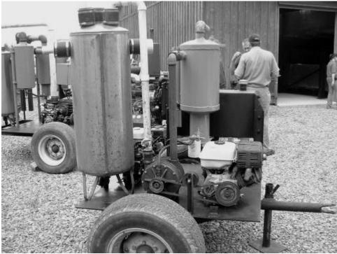
Gas powered vacuum pump on a trailer
