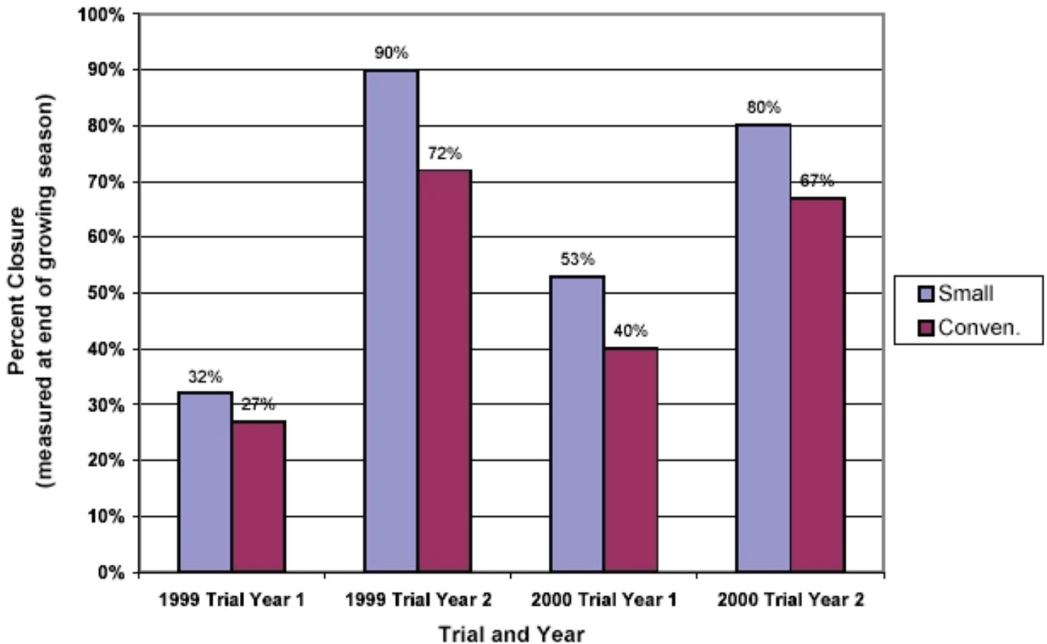
Taphole closure rate. Trees were tapped in 1999 (Treatment 1) and 2000 (Treatment 2), and tapholes were measured at the end of each growing season for both treatments. A completely closed taphole would measure 100%, and a wide open taphole would measure 0%. Small tapholes had closed more completely than large tapholes at the end of each growing season.
