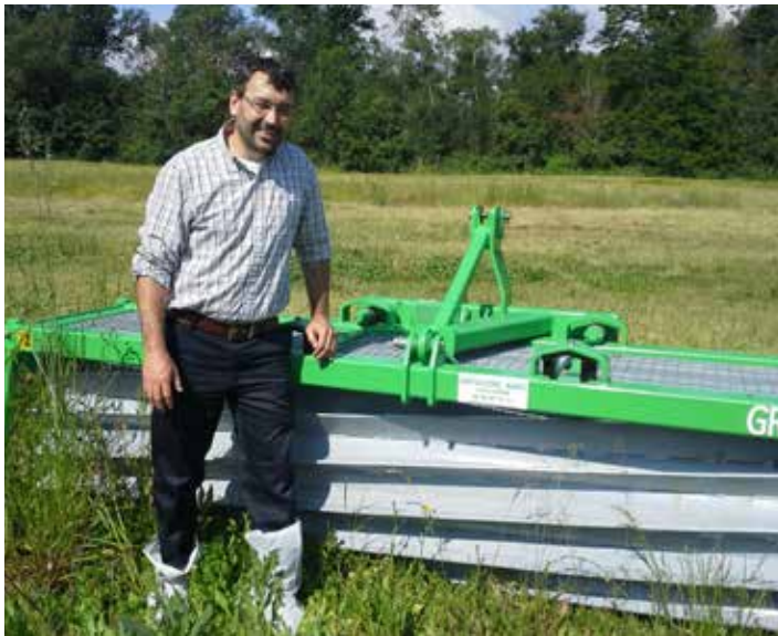
Figure 14. A roller-crimper in France with a reversible 3-point hitch that can be front or rear-mounted (top left). The blade on this front-mounted I & J roller-crimper is designed with a chevron pattern to minimize bouncing. The guard over the bearing prevents mulch residue from bunching up (bottom left). Rolling test strips in Penn Yan, NY. Adapters are available that allow attaching a roller-crimper to front loaders (right).
