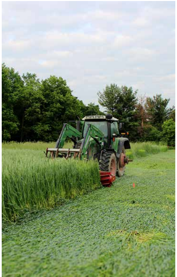
Figure 14. A roller-crimper in France with a reversible 3-point hitch that can be front or rear-mounted (top left). The blade on this front-mounted I & J roller-crimper is designed with a chevron pattern to minimize bouncing. The guard over the bearing prevents mulch residue from bunching up (bottom left). Rolling test strips in Penn Yan, NY. Adapters are available that allow attaching a roller-crimper to front loaders (right).
