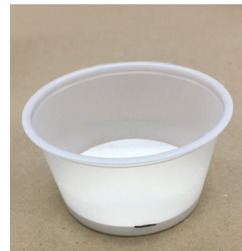
Portion cup marked at \frac{1}{4} inch with plaster mixture poured in.
