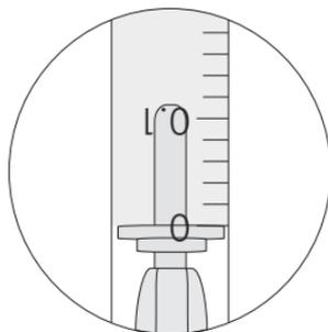
**NOTE:** When filling the Titrator from a container without a special plug, submerge the adapter tip below the surface of the solution and pull out the plunger. Remove air bubbles.
